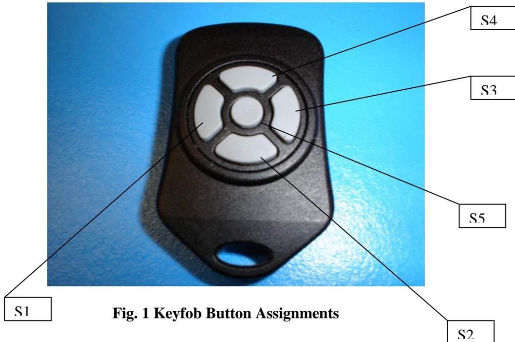
The RF-5000 comes in different configurations. Shown above is the 5-output example. This is the maximum controlled output using a keyfob. As the number of available outputs decreases so will the number of buttons on the keyfob.
